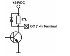
a) OC Internal circuit diagram
