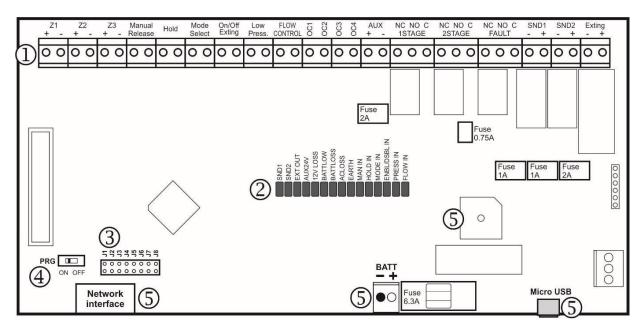
Figure 7 - Main PCB of FOT-IVY control panel
