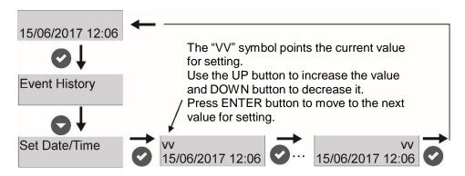
Set in sequence the current date, month and year, and time [Hour:Minutes]. After the last confirmation the module exits to normal operation mode.
