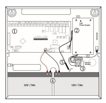
Figure 6 – Configuration of the modules in the box
